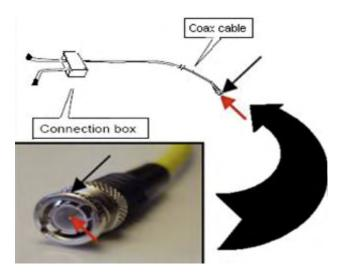
If you measure another value, unsolder the detection loop wires from the Connection box and replace the Connectionbox and coax cable. Measure the detectionloop before soldering. How to execute this process can be found in the ProChip Loop test step by step guide.
